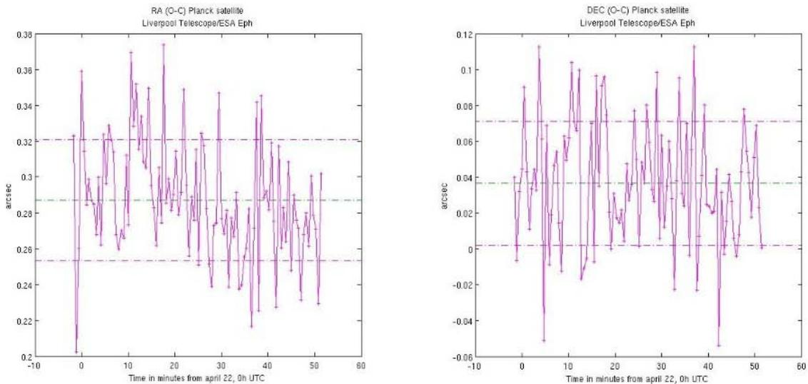
**Fig. 1** – Set of observations of the Planck satellite obtained with the 2 m Liverpool telescope with RATCAM reduced with the GBOT pipeline. Shown are the O-C (i.e observation vs. Ephemeris) residuals versus time. The R.M.S. Error in both coordinates is about 35 mas. UCAC2 (Zacharias et al. 2002) was used as reference catalog.
