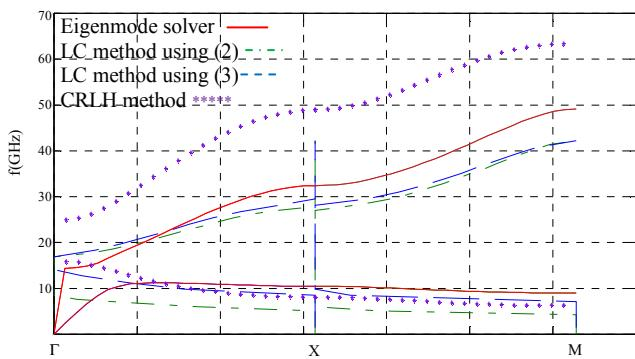
Figure 4. Comparison of dispersion diagram for  $W=2.25\text{mm}$ ,  $a=2.4\text{mm}$ ,  $h=1.6\text{mm}$ ,  $r=0.15\text{mm}$ ,  $\epsilon_r = 2.2$
