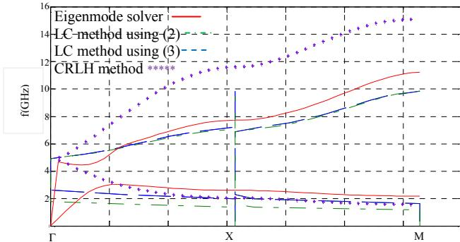
Figure 3. Comparison of dispersion diagram for  $W=9.6\text{mm}$ ,  $a=10\text{mm}$ ,  $h=3.08\text{mm}$ ,  $r=0.125\text{mm}$ ,  $\epsilon_r = 2.33$
