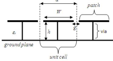
Figure 1. Side view of mushroom structure unit cell.
