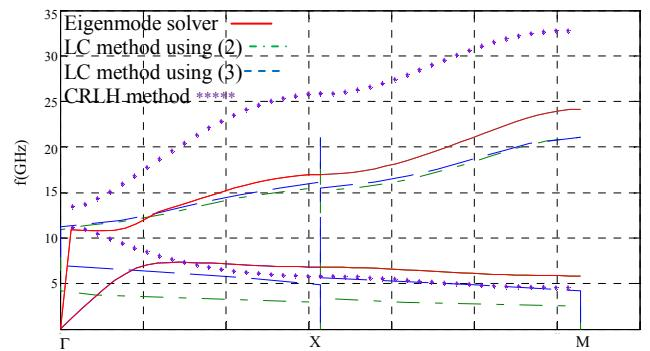
Figure 5. Comparison of dispersion diagram for  $W=4.5\text{mm}$ ,  $a=4.8\text{mm}$ ,  $h=1.6\text{mm}$ ,  $r=0.2\text{mm}$ ,  $\epsilon_r = 2.2$
