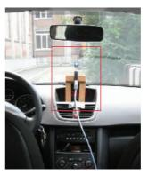
(a) Front Antenna (TX). The TX was placed in the center of the dashboard
