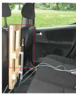
(b) Backside Antenna (RX). The RX was placed at a fixed position behind the driver's seat
