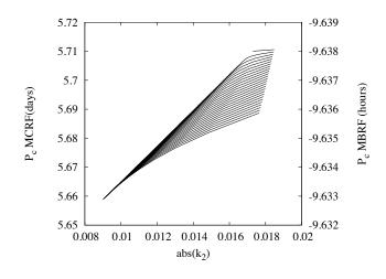
Fig. 5. Period of the Chandler model as a function of the value of the Love number  $k_2$ . The lower bound of  $k_2$  corresponds to a fully frozen model while the upper bound is expected if Ceres contains a global ocean.
