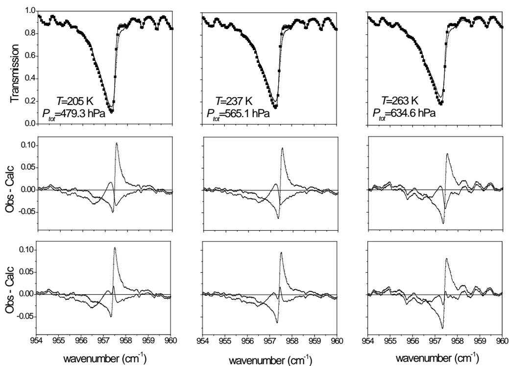
**Figure 3.** Comparison between measured transmissions ( $\bullet$ ) of  $\text{CH}_3\text{Br}$  diluted in  $\text{N}_2$  in the  $\nu_6$   $^RQ_0$  region and calculations without (---) (Lorentz lineshapes) and with (—) line-mixing effects using direct calculation (Eq. (1)). The corresponding residuals are plotted in the middle panels. For comparison, residuals with calculations using Lorentz (---) and Rosenkranz (—) profiles (Eqs. (9,10)) are shown in the lower panels.
