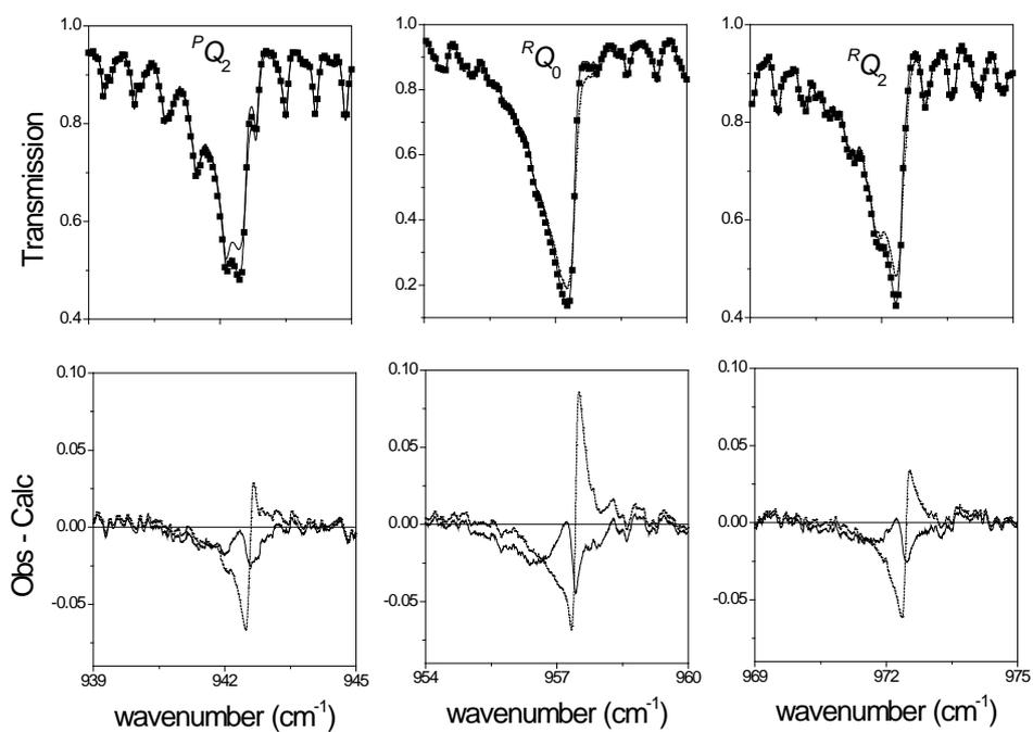
**Figure 4.** Comparisons for different branches between the calculations without (---) (Lorentz lineshapes) and with (—) taking into account line mixing effect (direct calculation). The experimental spectrum (■) corresponds to  $T=265$  K,  $P_{\text{CH}_3\text{Br}}=1.74$  hPa, and  $P_{\text{tot}}=545.50$  hPa.
