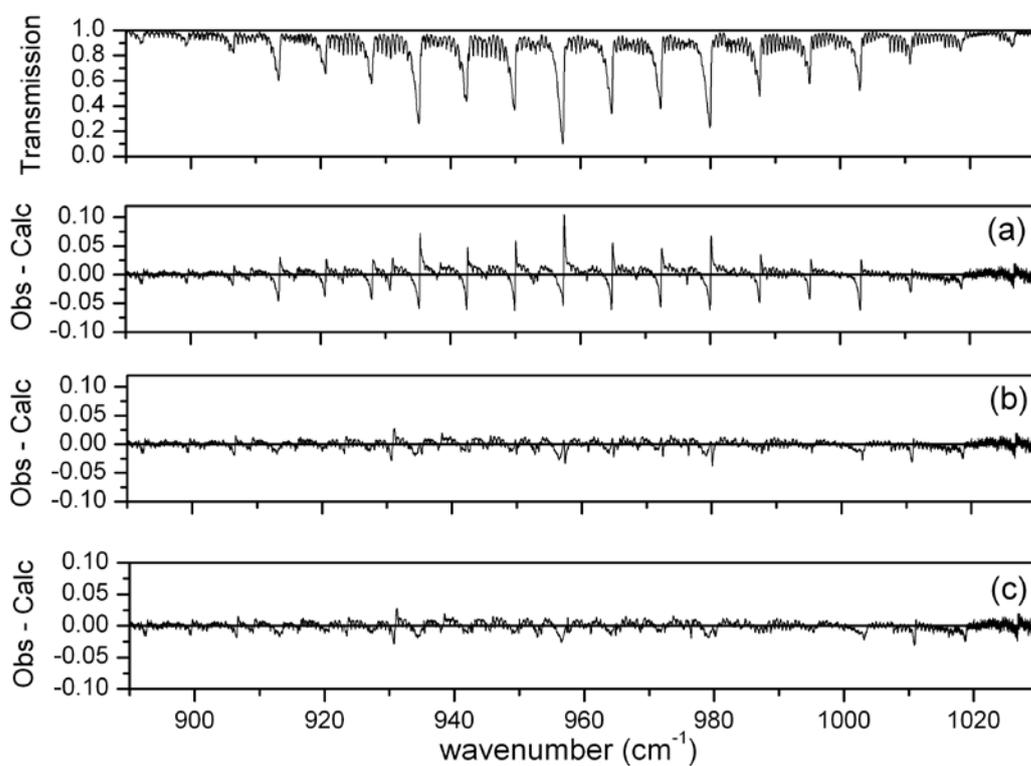
**Figure 1.** Overview of the  $\nu_6$  band for the experimental spectrum of  $\text{CH}_3\text{Br}/\text{N}_2$  at  $T = 234$  K ( $P_{\text{CH}_3\text{Br}} = 1.52$  hPa and  $P_{\text{tot}} = 476.1$  hPa). The residuals (obs-calc) have been plotted in the lower panels using Lorentz lineshapes (a), direct calculation of the relaxation operator (b), and Rosenkranz profile (c).
