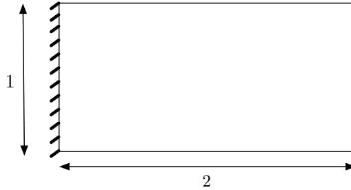
FIGURE 8. Boundary conditions for the long cantilever.
