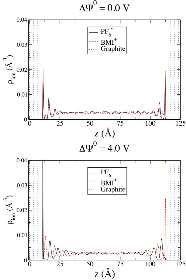
Figure 5: Ionic densities of anions and mass centers of cations for  $\Delta\Psi^0 = 0.0$  V and  $\Delta\Psi^0 = 4.0$  V. When the potential difference is not equal to 0.0 V, an asymmetry can be seen for the positive and negative electrodes.
