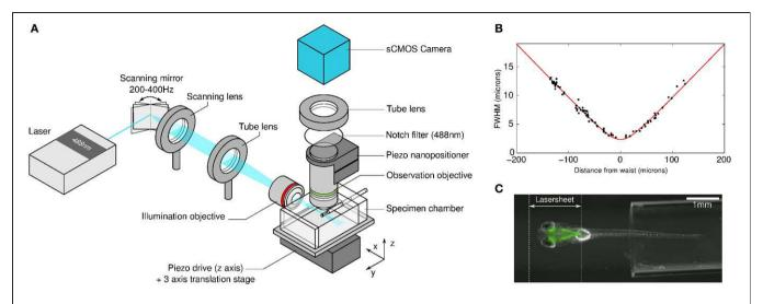
**FIGURE 1 | SPIM-based functional imaging. (A)** Sketch of the optical set-up. **(B)** Laser sheet thickness profile (FWHM) along the light propagation axis. Each data point corresponds to a measurement obtained with one fluorescent bead. The red curve is the best fit of the data with the theoretical
