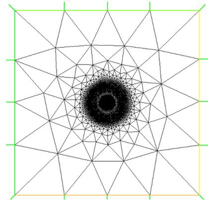
FIGURE 7. Mesh refinement for  $\gamma = 0.01$  : 9963 vertices
