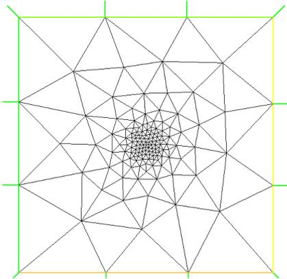
FIGURE 4. Mesh refinement for  $\gamma = 0.01$  : 148 vertices
