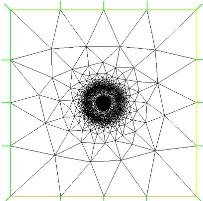
FIGURE 6. Mesh refinement for  $\gamma = 0.01$  : 5083 vertices
