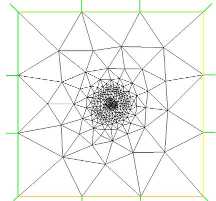
FIGURE 5. Mesh refinement for  $\gamma = 0.01$  : 334 vertices
