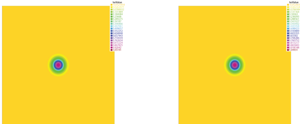
FIGURE 11. Exact solution (left) and numerical solution (right) after the mesh refinement for \lambda = 10 and p = 1 .
