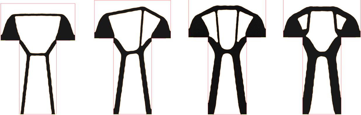
FIGURE 10. (From left to right): Optimal shapes of a mast for compliance minimization, with uncertainties on the body forces of amplitude  $m = 0, 0.6, 2, 3$ . The same Lagrange multiplier for the volume constraint is used in all cases.
