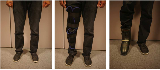
Fig. 7. Mechanical disturbances on the subject: normal (left), right knee immobilization (center) and ski boot on right foot (right)
