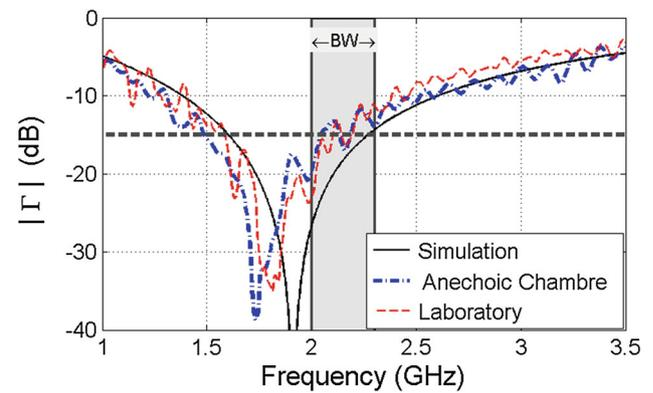
Fig. 7 Comparison between simulation and measurements results at normal incidence ( $d_a = 8$  cm,  $d_{am} = 107$  cm)
