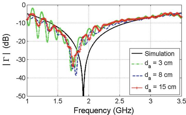
**Fig. 9** Influence of the distance between Tx and Rx Antennas ( $d_a$ ) on the reflection coefficient (at normal incidence and with  $d_{am} = 107$  cm)
