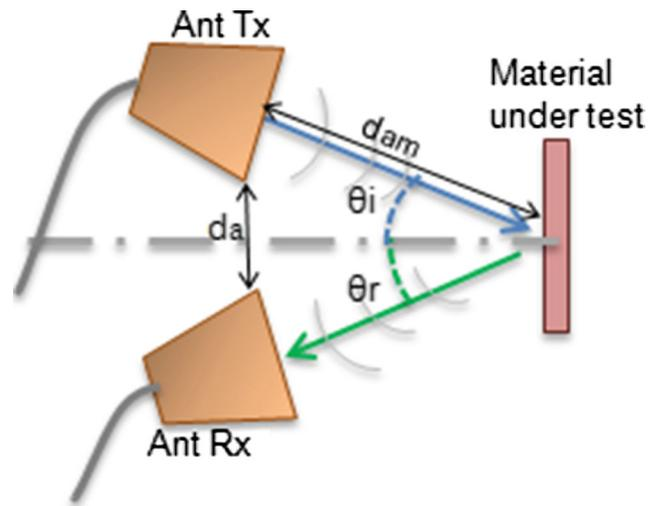
Fig. 6 Measurement setup at oblique incidence
