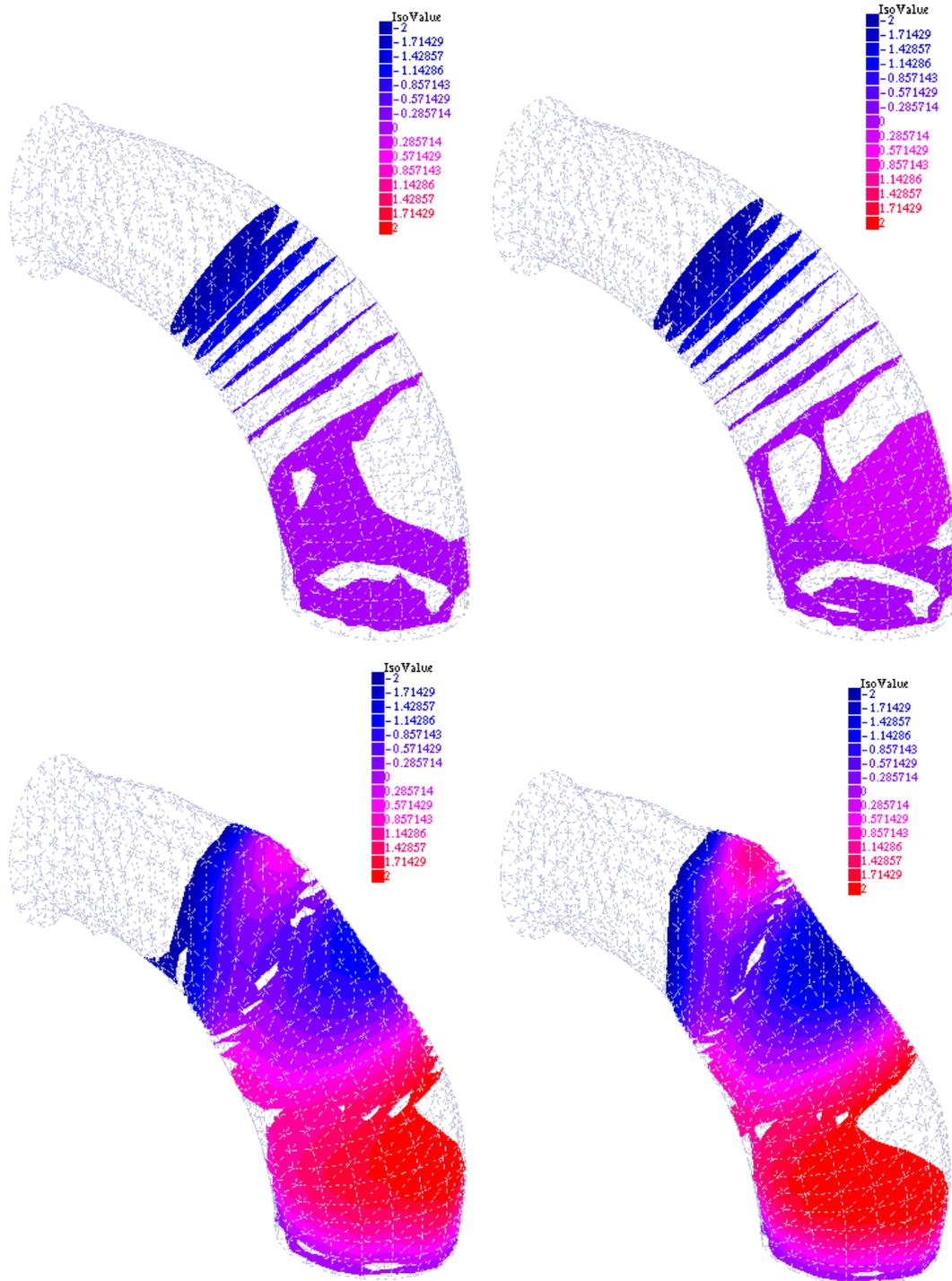
Figure 1: Surface of equal pressure at  $t = 0.8$ . Top left: computed by solving (63) with Euler's scheme. Top right: computed by solving (65) with Euler's scheme. Bottom left: computed by solving (63) with Crank-Nicolson's scheme. Bottom right: computed by solving (65) with Crank-Nicolson's scheme.
