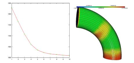
Figure 3: Left: Optimization criteria  $\int_{\Sigma \times (0,T)} p^4$  versus iteration number. Right: the coefficient b(x) after 4 iterations. Right: effect of the change of b on the dilatation of the vessel.
