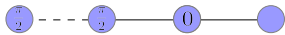
FIG. 2: A MBQC scheme where a Fourier transform is implemented on an input state by attaching it to a linear cluster state and by performing measurements on the cluster modes.
