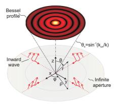
Fig. 1. Schematic view of the considered configuration. The aperture field distribution is a cylindrical inward wave with radial propagation constant  $k_{\rho a}$ . The non-diffractive zone is limited by the cone with angle  $\theta_a = \sin^{-1}(k_{\rho a}/k)$ , where k is the free space wavenumber.
