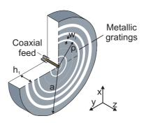
Fig. 6. Radial waveguide loaded with metallic gratings and fed by a coaxial fed.
