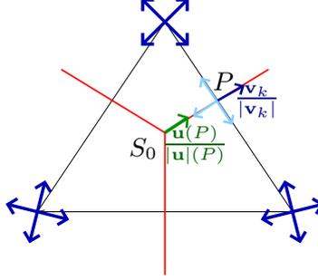
**Fig. 4.** The intersection of a separatrix (in red) of the singularity  $S_0$  with the triangle around  $S_0$ , at a point  $P$ .
