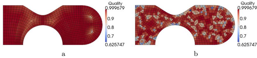
**Fig. 8.** Color map of the Jacobian quality measure on our mesh (in a) and on the unstructured mesh (in b) as a color map.
