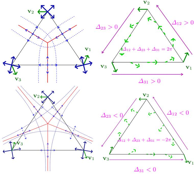
**Fig. 6.** A 3-valent singularity, on top, and a 5-valent singularity, on bottom. In blue, the local cross field, and in green the corresponding representation vector field. Separatrices are in red, along with the shape of surrounding streamlines in blue dots. On the right, in light green dots, the linear interpolation of the representation vectors along the edges is shown. The path along which we compute the index is the triangle around the singularity.
