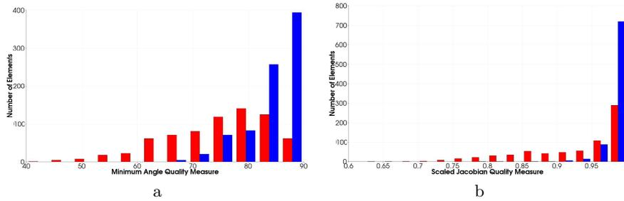
**Fig. 9.** Histograms representing the repartition of elements by quality, the unstructured mesh being represented in red and our mesh in blue. In (a) the histogram represents the repartition for the minimum angle quality, and in (b) it represents the repartition for the Jacobian quality.
