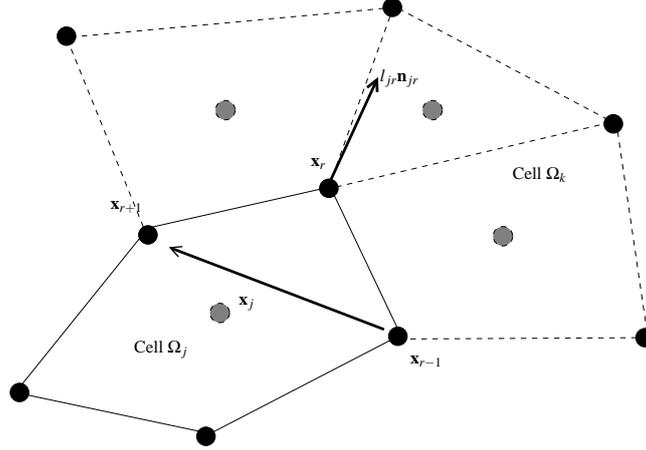
Figure 5: Notation for nodal formulation: the corner length  $l_{jr}$  and the corner normal  $\mathbf{n}_{jr}$ . Notice that  $l_{jr} \mathbf{n}_{jr}$  is equal to the orthogonal vector to the half of the vector that starts at  $\mathbf{x}_{r-1}$  and finish at  $\mathbf{x}_{r+1}$ . The center of the cell is an arbitrary point inside the cell.
