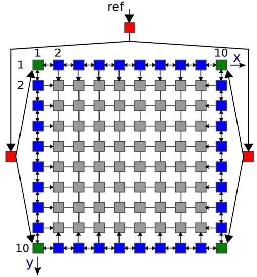
Fig. 3. Proposed network topology ( $\rightarrow$ : unidirectional;  $\leftrightarrow$ ,  $-$ : bidirectional)
