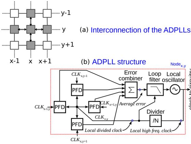
Fig. 1. Interconnection and structure of the ADPLLs
