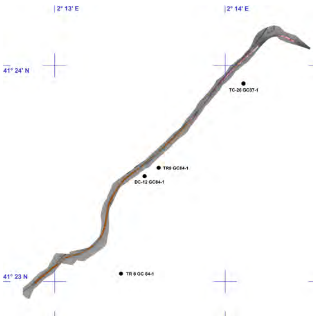
Fig. 20 Location of cores and grabs (see Appendix) superimposed on backscattering image and segmentation map of West-Besos.
