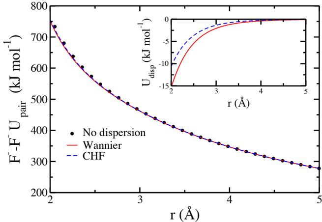
FIG. 1: Sum of the three pairwise additive terms for the  $F^-$ - $F^-$  interaction (inset: dispersion term only). The distance range corresponds to the extent of the first peak of the  $F$ - $F$  partial radial distribution function in liquid  $LiF$  (shown in Figure 2).
