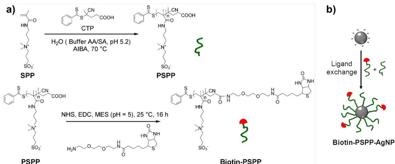
**Fig. 1.** Elaboration of the electrochemical label. (a) Synthesis of zwitterionic polymers, PSPP by RAFT polymerization and biotin-PSPP by coupling of PSPP with amino-PEG<sub>2</sub>-biotin. (b) ligand exchange procedure using a mixture of PSPP and Biotin-PSPP on 13 nm diameter silver nanoparticles.
