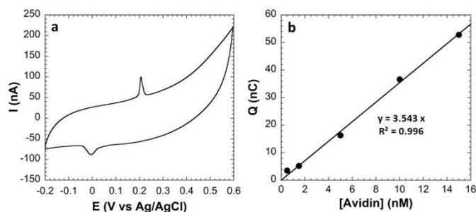
**Fig. 3** (a) Cyclic voltammogram on Au/Biotin/Avidin/Biotin-PSPP-AgNP in 0.1 M PBS pH 7.0 solution at a scan rate of  $50 \text{ mV s}^{-1}$ , [Avidin] = 5 nM. (b) Calibration curve of the relationship between oxidation charge of AgNP and avidin concentration used in sandwich elaboration.
