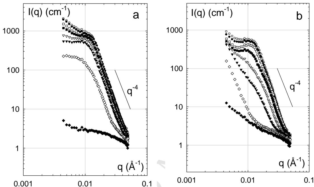
**Figure 7.** Double logarithmic plots of the scattering intensity of 8 wt% PN-D (a) and PD-N (b) solutions at different temperatures ( $T$  °C): 29.0 (◆), 33.0 (◇), 35.0 (▼), 36.0 (▽), 38.5 (■), 43.0 (□), 51.0 (●) and 57.5 (○).
