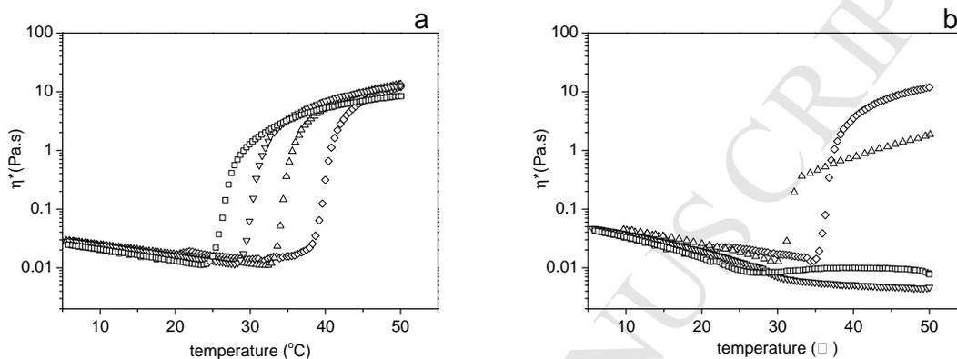
**Figure 11.** Influence of salt on viscoelastic properties of PD-N (a) and PN-D (b) aqueous solutions ( $C_p=3$  wt%,  $f=1$  Hz, heating rate= $2$  °C/min).  $K_2CO_3$  concentrations: 0 ( $\diamond$ ), 0.1 ( $\triangle$ ), 0.2 ( $\nabla$ ) and 0.3 mol/L ( $\square$ ).
