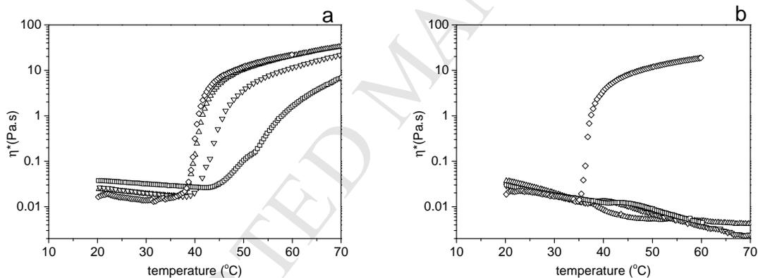
**Figure 13.** Influence of SDS on viscoelastic properties of PD-N (a) and PN-D (b) aqueous solutions ( $C_p=3$  wt%,  $f=1$  Hz, heating rate= $2$  °C.min $^{-1}$ ). SDS concentrations: 0 ( $\diamond$ ), 2 ( $\triangle$ ), 5 ( $\nabla$ ) and 10 mM ( $\square$ ).
