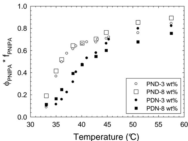
**Figure 8.** Temperature dependence of the PNIPA-rich phase with  $f_{\text{PNIPA}}$  the fraction of PNIPA embedded in the segregated phase and  $\phi_{\text{PNIPA}}$  their volume fraction estimated from the SANS invariant analysis .
