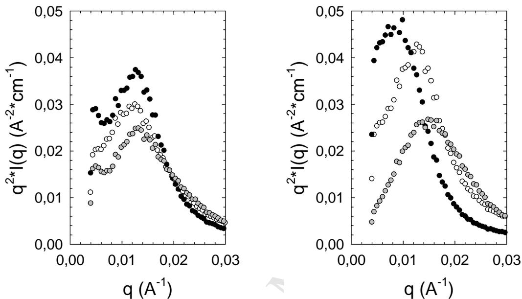
**Figure S6.** SANS patterns of PD-N (left) and PN-D (right) copolymers at 3 wt % in water (○),  $K_2CO_3$  0.3 M (●) and SDS 2.5 mM (●). All the experiments have been performed at high temperature :  $T = 57$  °C.
