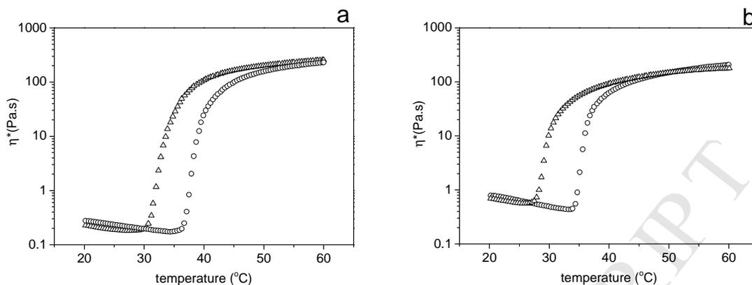
**Figure S7.** Influence of salt on viscoelastic properties of PD-N (a) and PN-D (b) aqueous solutions ( $C_p=10$  wt%,  $f=1$  Hz, heating rate= $2$  °C.min $^{-1}$ );  $[K_2CO_3] = 0$  mol/L (○) and  $0.3$  mol/L (△)
