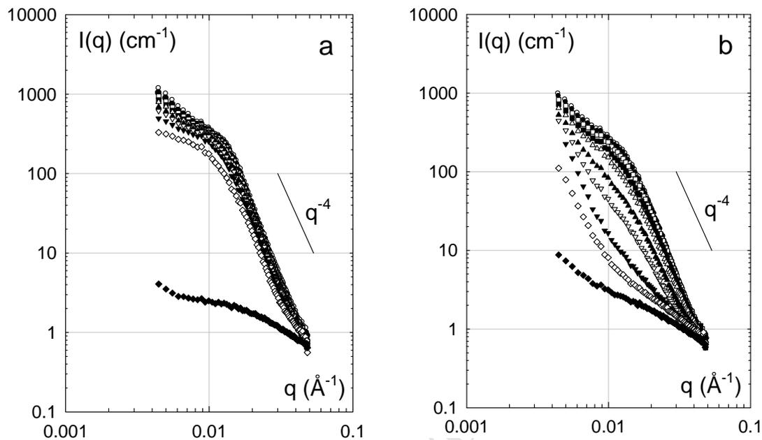
**Figure 6.** Double logarithmic plots of the scattering intensity of 3 wt% PN-D (a) and PD-N (b) solutions at different temperatures ( $T$  °C): 33.0 (◆), 35.0 (◇), 36.0 (▼), 37.0 (▽), 38.5 (▲), 40.0 (△), 43.0 (■), 45.5 (□), 51.0 (●) and 57.5 (○).
