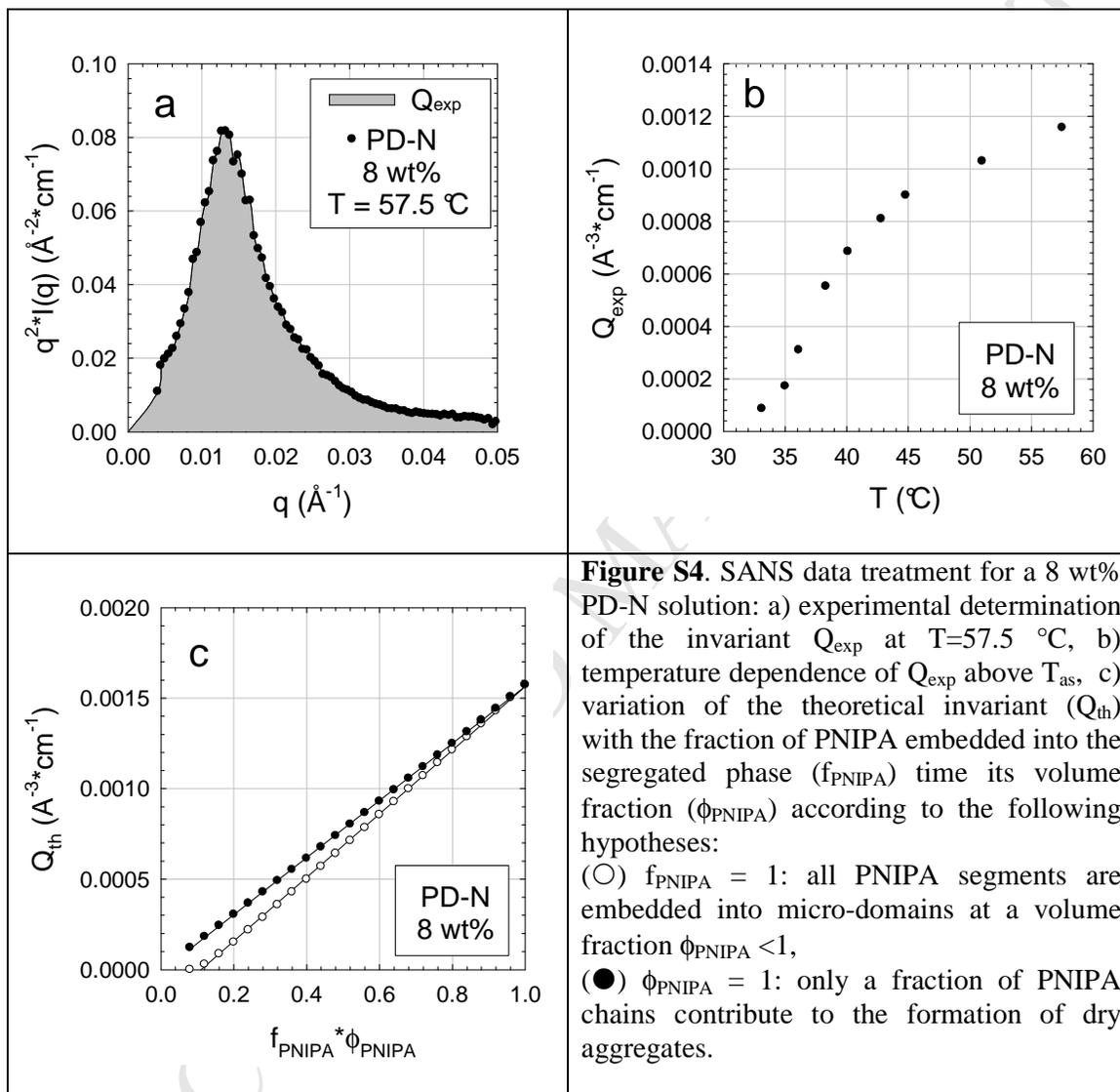
The determination of  $Q_{\text{exp}}$  as a function of temperature (see **Figure S4b**) can be used to determine the fraction of PNIPA embedded in the segregated phase ( $f_{\text{PNIPA}}$ ) time their volume fraction ( $\phi_{\text{PNIPA}}$ ) according to two different hypotheses:
