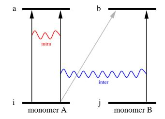
FIG. 1. Single excitations (arrows) between an occupied (i or j) and a virtual (a or b) orbital in two monomers. These single excitations can either be intra-molecular (black arrows) or inter-molecular (gray arrow). One can then consider the coupling of two intra-molecular single excitations either within the same monomer (red double wavy line) or between two monomers (blue wavy line). These last couplings we call 'dispersion-type combination of intra-monomer excitations'.
