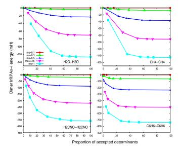
FIG. 2. Evolution of the lrRPAx-I dimer energies (in mH) with the number of selected determinants (in % of the possible determinants) for thresholds of  $10^{-5}$ ,  $10^{-6}$ ,  $10^{-7}$ ,  $10^{-8}$ ,  $10^{-9}$ ,  $10^{-10}$  Hartrees (from left to right, as tighter thresholds select more determinants) for the water (top left), the methane (top right), the formamide (bottom left) and the benzene dimer (bottom right).
