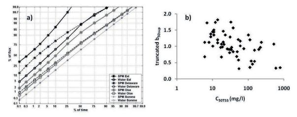
**Fig. 3** (a) River flows and sediment fluxes duration curves represented in double probability scales. Mid-latitude basins of similar size: Eel and Delaware (USA) and Oise and Somme (France) rivers (Moatar *et al.*, 2013, *Hydrol. Processes*, reproduced with permission). (b) Truncated rating curve exponent (b<sub>50sup</sub>) vs median TSS in world rivers.
