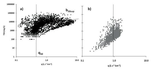
**Fig. 4** Truncated rating curve between TSS and river flow in the Colorado River at Grand Canyon (AZ; USGS ID 09402500): (a) prior to the damming impact (1931–1941); (b) afterwards (1964–1971). See Table 1 for related variability metrics.
