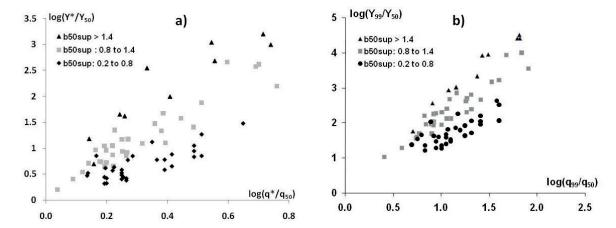
**Fig. 6** Daily TSS flux variability vs daily flow variability for three classes of  $b_{50sup}$ : (a) General flux variability  $(Y^*/Y_{50})$  vs general flow variability  $(q^*/q_{50})$ ; (b) Extreme flux variability  $(Y_{99}/Y_{50})$  vs extreme flow variability  $(q_{99}/q_{50})$ ; log-log scales.
