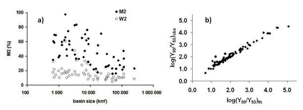
**Fig. 2** Range of duration and of extreme sediment flux characteristics in world rivers: (a) Flow duration  $(W_2)$  and sediment flux duration  $(M_2)$  in 2% of time vs river basin size. (b) Observed extreme variability for daily yields  $(Y_{99}/Y_{50})$  vs theoretical variability (Meybeck *et al.*, 2003; Meybeck & Moatar, 2012).
