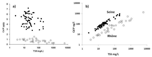
Fig. 10 Cadmium control by TSS in Seine and Rhone Rivers (France): (a) Cd contents ( $\mu$ g/g or ppm) in suspended particulates  $\nu$ s TSS; (b) calculated total cadmium concentration (ng Cd/L)  $\nu$ s TSS.
