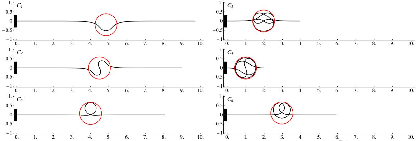
Figure 6: Post-buckling configurations. Top row shows  $Ax$  configurations, symmetric with respect to the axis joining the center of the disk  $(x_C, y_C)$  and the beam midpoint  $(x(\ell/2), y(\ell/2))$ . Middle row shows  $Pt$  configurations, symmetric with respect to the beam midpoint  $Pt$ . Bottom row represents  $L_1$  and  $L_2$  configurations. The circles have center  $(x_C, y_C)$  and radius  $(1 + \rho)/2$ .
