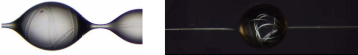
Figure 1: Experiments on fibers bent inside liquid drops. Left: microscopic photograph of spider capture silk. Flagelliform core filaments are seen to be coiled and packed inside a (typically  $300 \mu$  wide) glue droplet. Right: same mechanism reproduced artificially with a  $200 \mu\text{m}$  synthetic droplet and fiber (see experimental verification section in section 4). Reproduced from [6].
