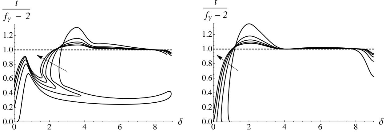
Figure 7: Equilibrium paths for  $f_\gamma = 10, 20, \dots, 50$  with the vertical axis rescaled according to Equation (14). (Left) Axis-symmetric ( $Ax$ ) configurations and (Right) Point-symmetric ( $Pt$ ) configurations. Direction of increasing  $f_\gamma$  is indicated with the arrows.
