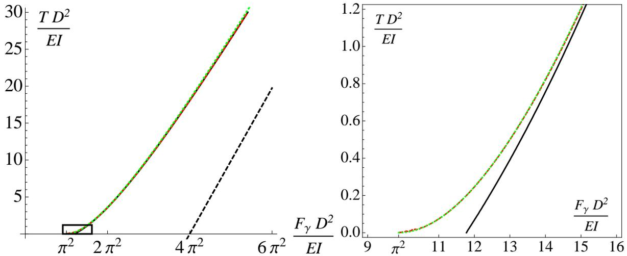
Figure 3: Buckling curve for  $\ell = 5$ . (Left) Curves defined by Equations (11) (12) (13). At this scale the three curves are almost indistinguishable. The asymptote  $t = f_\gamma - 4\pi^2$  is shown dashed. (Right) Zoom corresponding to the rectangle shown on the Left. The approximations (12) (13) are still hard to distinguish, but are seen to deviate from the exact curve (11), shown continuous and black.
