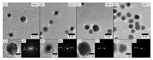
Figure 5: HRTEM images of  $(Co_{30}Pt_{70})_{Polyol}$  at various annealing temperatures: (A) 300°C; (B) 420°C; (C): 550°C and (D) 680°C. For each temperature, HRTEM images of one nanoparticle (A2, B2, C2, D2) and the associated FFT (A3, B3, C3, D3).
