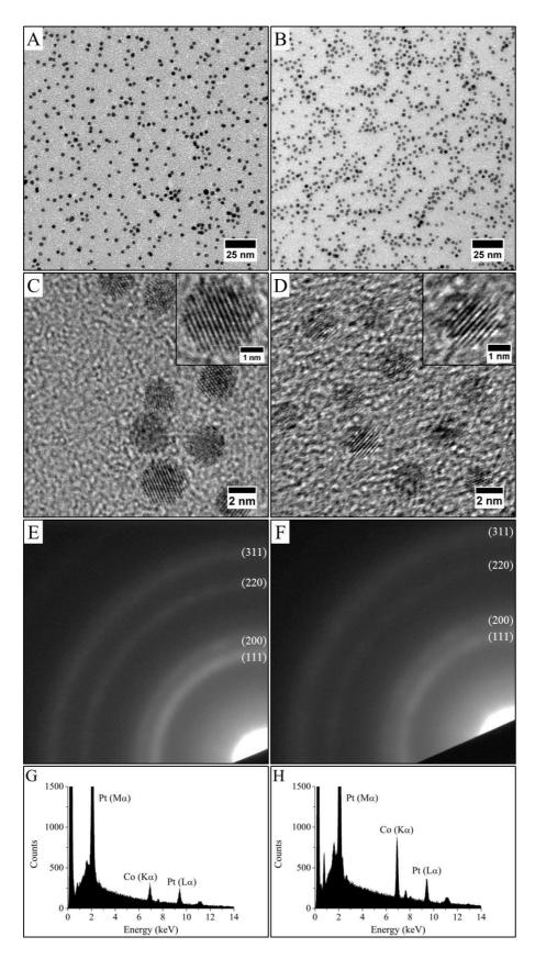
Figure 2: TEM images (A-B), HRTEM images (C-D), electronic diffraction (E-F) and EDX analysis (G-H) of (Co<sub>30</sub>Pt<sub>70</sub>)<sub>Polyol</sub> (left images) and (Co<sub>50</sub>Pt<sub>50</sub>)<sub>Polyol</sub> (right images).
