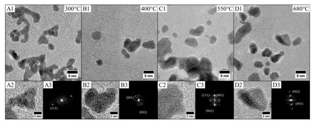
Figure 7: HRTEM images of  $(Co_{30}Pt_{70})_{LLPT}$  at various annealing temperatures: (A) 300°C; (B) 400°C; (C): 550°C and (D) 680°C. For each temperature, HRTEM images of one nanoparticle (A2, B2, C2, D2) and the associated FFT (A3, B3, C3, D3).
