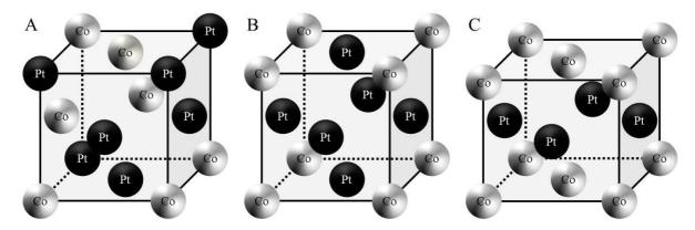
Figure 1 : Representation of  $Co_X Pt_{100-X}$  structure in three different phases: (A) disordered phase A1 with cubic symmetry (B) ordered phase  $L1_2$  with cubic symmetry (X=25) and (C) ordered phase  $L1_0$  with face centered tetragonal symmetry (X=50).
