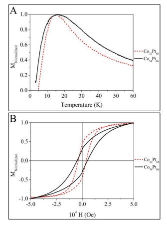
Figure 4: (A) Temperature dependence of the magnetization in the Zero-Field Cooled curves with applied field H=100 Oe and (B) hysteresis loop of  $(Co_{30}Pt_{70})_{Polyol}$  (dash line) and  $(Co_{30}Pt_{70})_{LLPT}$  (solid line).
