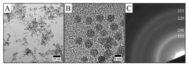
Figure 3: TEM images (A), HRTEM images (B) and electronic diffraction (C) of (Co<sub>30</sub>Pt<sub>70</sub>)<sub>LLPT</sub>
