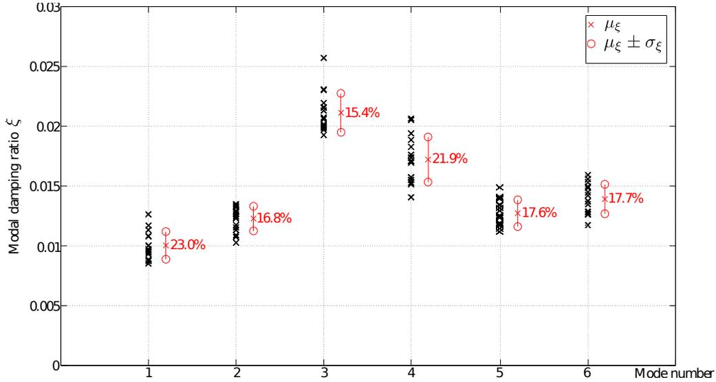
Figure 13: (colours online only) Identified modal damping ratios for the 17 *Type-1* specimens. For each mode, the black crosses indicate the single modal damping ratios. For each mode, the red crosses indicates the mean value  $\mu_\xi$  of the 17 modal damping ratios. The red circles indicate the spread of the modal damping ratios around the mean value, as 1 standard deviation below and above the mean value:  $\mu_\xi \pm \sigma_\xi$ . Red numbers indicate the value  $\sigma_\xi / \mu_\xi$ .
