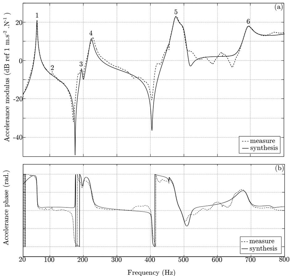
Figure 5: Sample *Type1* guitar (tendencies are the same for the sample *Type 2* guitar): modal identification with the LSCF method implemented in the software MODAN. (a) modulus, (b) phase. The dashed line curve is the measured accelerance, the solid line curve is the synthesised acceleration. A mode numbering is indicated. The mode 2 is identified separately. The mode near 500 Hz is a mode that does not involve the neck, so it is not numbered.
