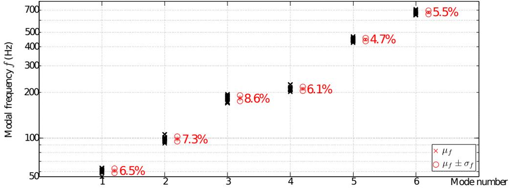
Figure 11: (colours online only) Identified modal frequencies for the 17 *Type-1* specimens. For each mode, the black crosses indicate the single modal frequencies. For each mode, the red crosses indicate the mean value  $\mu_f$  of the 17 modal frequencies. The red circles indicate the spread of the modal frequencies, as 1 standard deviation below and above the mean value:  $\mu_f \pm \sigma_f$ . Red numbers indicate the value  $\sigma_f/\mu_f$ .
