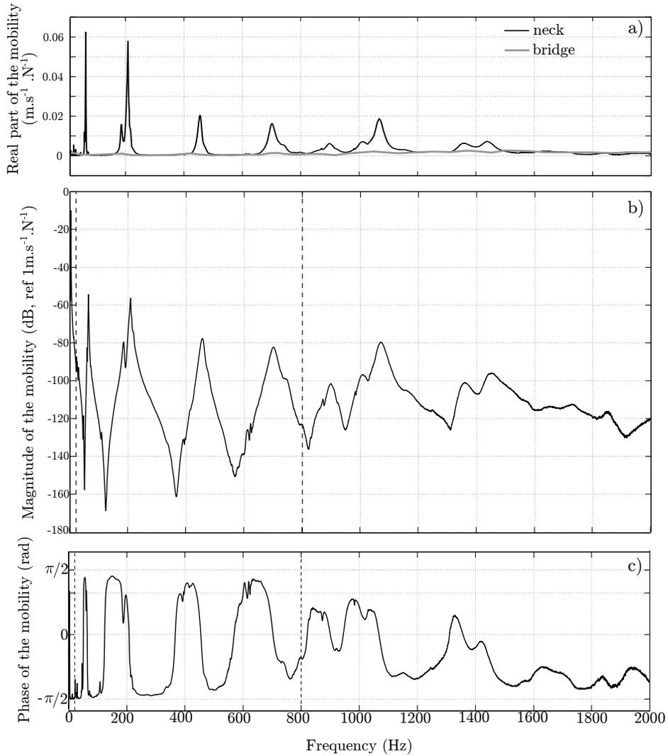
Figure 1: Driving point mobility measurement on the neck of one *Type-2* guitar. a) Real part (conductance, in  $\text{m.s}^{-1}.\text{N}^{-1}$ ), for comparison purposes, the gray line presents the conductance measured at the bridge. b) Magnitude in dB scale normalised to  $1 \text{ m.s}^{-1}.\text{N}^{-1}$ . c) Phase. The thick black dashed lines indicate the frequency bandwidth of the study [20 Hz : 800 Hz].
