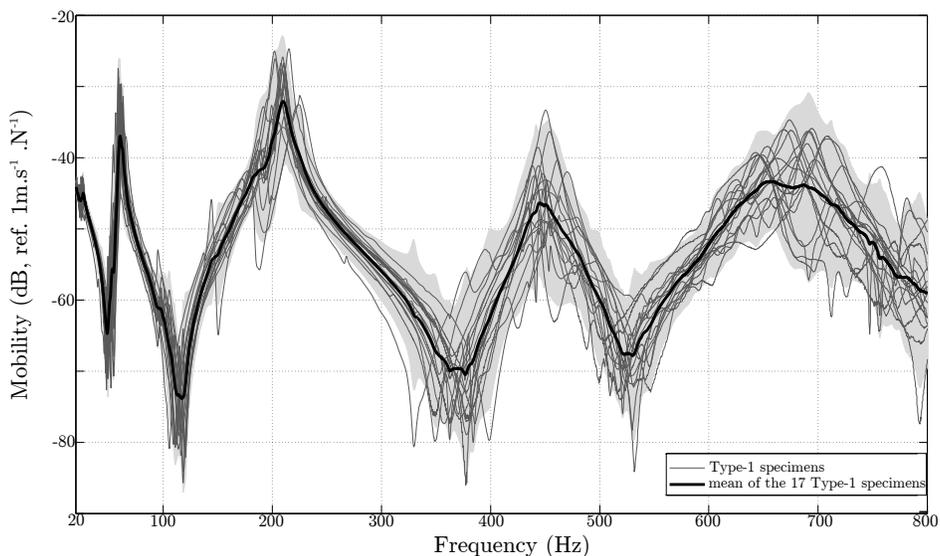
Figure 6: Superimposition of all mobility curves for the 17 *Type-1* specimens. Individual mobility curves are represented with thin gray lines. The thick black line is the mean mobility. The gray area is centered on this mean mobility, and its boundaries are two standard deviation below and above the mean mobility.
