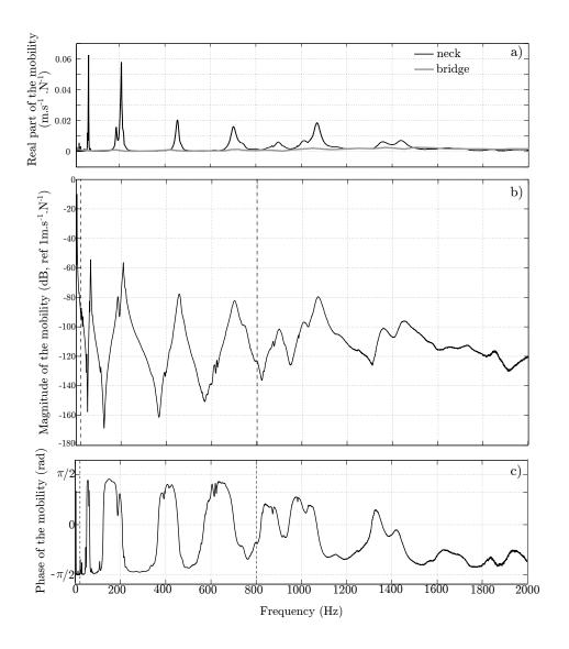
Figure 1: Driving point mobility measurement on the neck of one Type-2 guitar. a) Real part (conductance, in  $m.s^{-1}.N^{-1}$ ), for comparison purposes, the gray line presents the conductance measured at the bridge. b) Magnitude in dB scale normalised to  $1 m.s^{-1}.N^{-1}$ . c) Phase. The thick black dashed lines indicate the frequency bandwidth of the study [20 Hz : 800 Hz].
