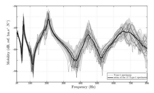
Figure 6: Superimposition of all mobility curves for the 17 *Type-1* specimens. Individual mobility curves are represented with thin gray lines. The thick black line is the mean mobility. The gray area is centered on this mean mobility, and its boundaries are two standard deviation below and above the mean mobility.
