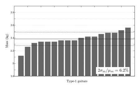
Figure 9: Bar plot of the masses of the 17 Type-1 guitars. The black solid line indicates the mean mass  $\mu_m$ . The black dotted lines indicate the spread around the mean mass as 1 standard deviation below and above the mean mass:  $\mu_m \pm \sigma_m$ . The 2-standard deviation spread around the mean is indicated as a percentage of the mean mass.
