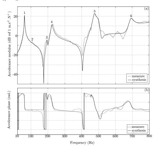
Figure 5: Sample *Type1* guitar (tendencies are the same for the sample *Type2* guitar): modal identification with the LSCF method implemented in the software MODAN. (a) modulus, (b) phase. The dashed line curve is the measured accelerance, the solid line curve is the synthesised accelerance. A mode numbering is indicated. The mode 2 is identified separately. The mode near 500 Hz is a mode that does not involve the neck, so it is not numbered.
