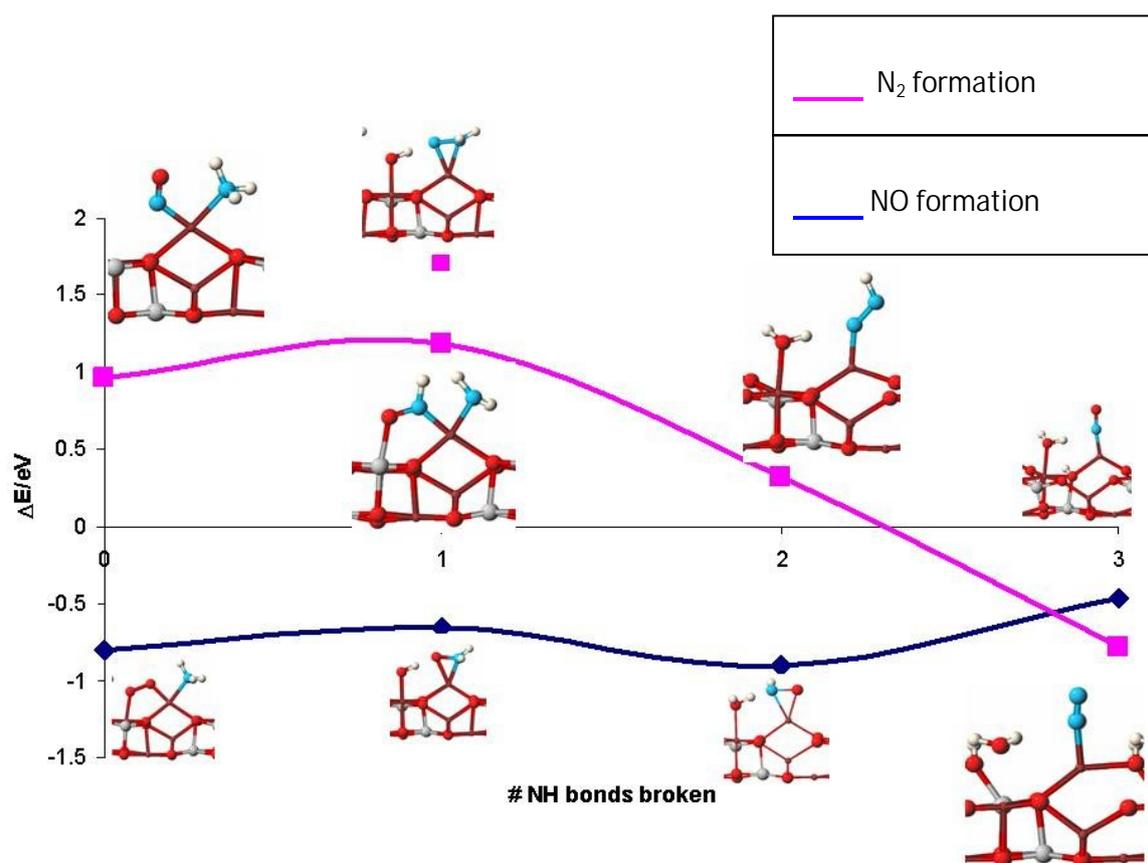
Figure 10: Different intermediates in the  $\text{NH}_3 + \text{NO}$  reaction, compared to the  $\text{NH}_3 + \text{O}_2$  reaction. The line of zero energy corresponds to the addition of the individual adsorption energies (no co-adsorption effect).
