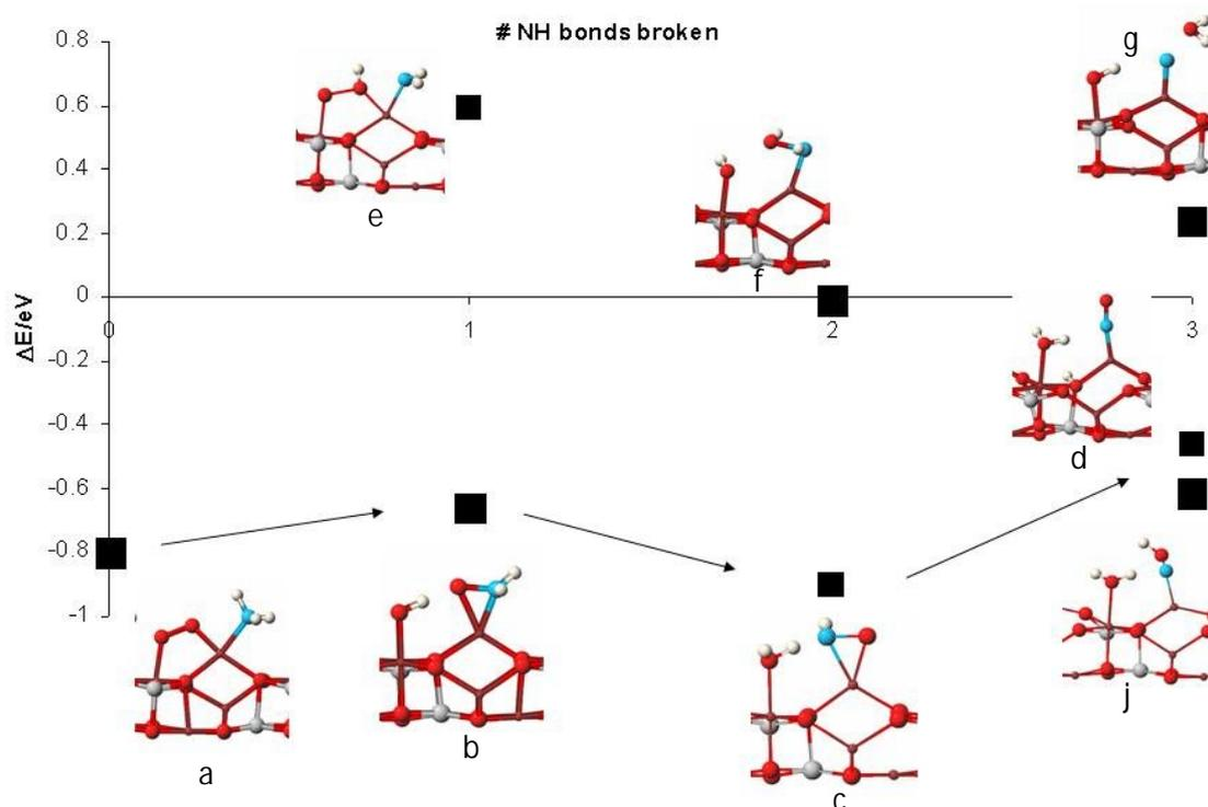
Figure 9: Different intermediates in the  $\text{NH}_3 + \text{O}_2$  reaction. The line of zero energy corresponds to the addition of the adsorption energies of  $\text{NH}_3$  and  $\text{O}_2$  (no co-adsorption effect).
