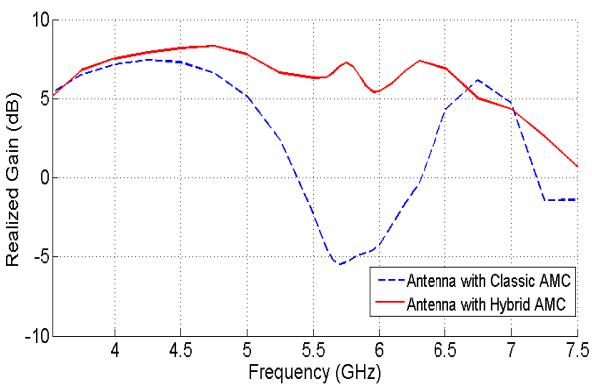
Fig. 5. Realized gain in broadside direction versus frequency.
