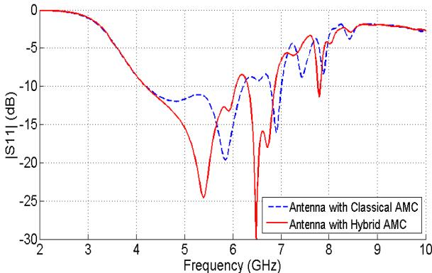
Fig. 4. Magnitude of reflection coefficient versus frequency.
