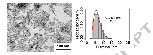
Figure 1: Left: TEM picture of the BNP; right: size distribution obtained by TEM pictures analysis (red line: log-normal distribution model, with  $d_0 = 6.1$  nm and  $\sigma = 0.33$ )
