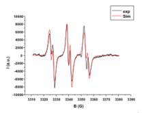
Figure 3. ESR spin trapping (PBN) spectrum. [PBN] =  $7.90 \cdot 10^{-4}$  M, [1] =  $1.57 \cdot 10^{-4}$  M, [2] =  $1.91 \cdot 10^{-3}$  M in 1.5 mL of DCM/*tert*-butylbenzene 1:2.
