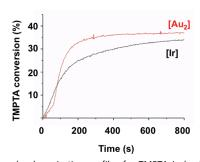
**Figure 4** Compared polymerization profiles for TMPTA in laminate system for different catalysts upon a blue LED bulb irradiation (405 nm). Red curve: 2/5/1 (1/100/0.0125 mol/mol); black curve: 2/5/fac-Ir(ppy)<sub>3</sub> (1/100/0.0125 mol/mol).
