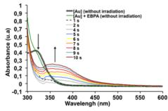
Figure 2 Steady state photolysis of  $\bf 1$  and  $\bf 2$  in dichloromethane upon exposure to the Xe-Hg under air at different irradiation times (from t=0 to  $\bf 10$  s).  $\bf 1/2$ :
