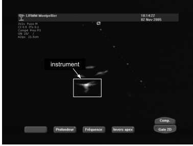
Fig. 8. Instrument image with 20 dB intensity gain
