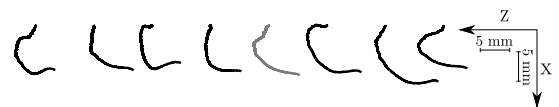
Fig. 6. Harpist forefinger movement during plucking actions. The grayed movement is used as reference for the robot.
