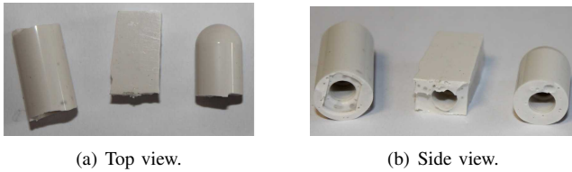
Fig. 4. Silicone fingertips of three different shapes: B-C-A
