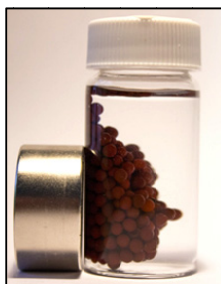
Figure 1: Photograph of the MagAlbeads attracted with a small permanent NdFeB magnet (diameter: 2.5 cm; height: 1cm).
