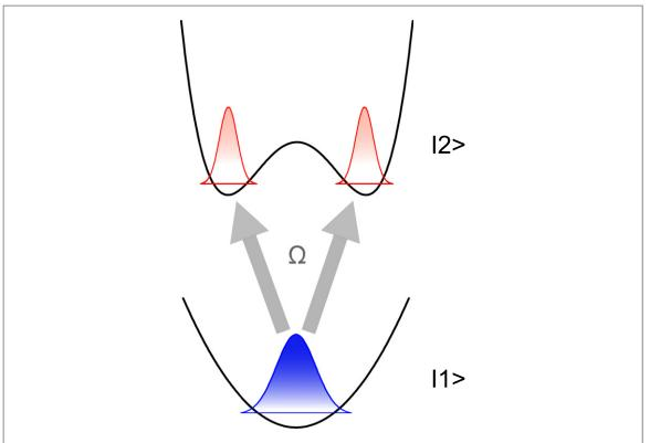
**Figure 1.** Schematics of the beam-splitter: atoms are transferred from a single to a double-well by coherently coupling (with Rabi frequency  $\Omega$ ) two long-lived internal states in the presence of a state-selective potential.
