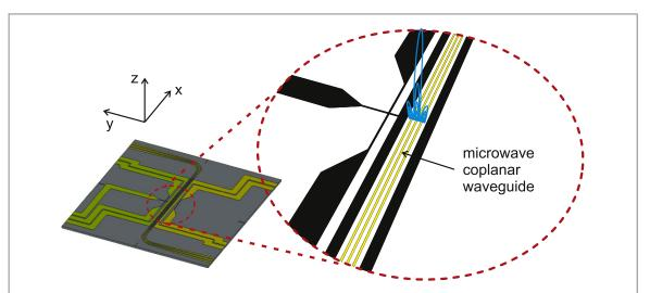
**Figure 5.** Schematics of the chip first layer. A zoom in the centre of the chip shows the three wires which form the microwave coplanar waveguide. The central wire of the CPW is used, in addition, to carry the stationary current for the generation of the magnetic trap. In the present realization the two side wires of the CPW are grounded at the chip.
