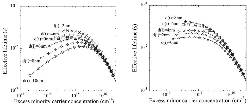
Fig. 4. Effective lifetime versus excess minority carrier concentration for several values of the (i)a-Si:H buffer layer thickness,  $d(i)$ , with a constant value of the valence band tail Urbach parameter,  $E_u$ , (Fig. 4a) and with a parabolic parameterization of  $E_u$  (Fig. 4b)
