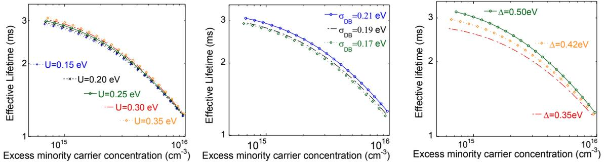
Fig. 2. Effective lifetime versus excess minority carrier concentration for several values of (a) the correlation energy  $U$ , (b) the standard deviation of the Gaussian pool  $\sigma_{DB}$ , and (c) the energy separation  $\Delta$ .
