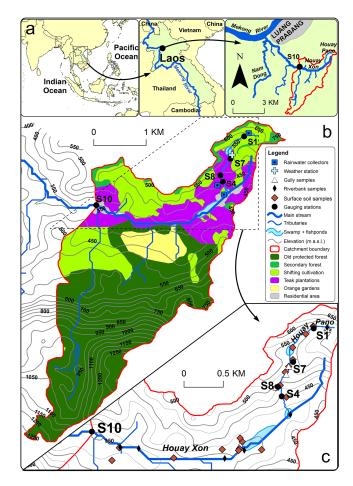
**Figure 1.** Location of the Houay Xon River catchment in SE Asia (a). Topographic and land use map of the Houay Xon S10 subcatchment in 2012 with location of the gauging stations (S1, S4, S7, S8, S10), rainwater collectors and automatic weather station (b), surface soil, gully and riverbank sampling locations (c).
