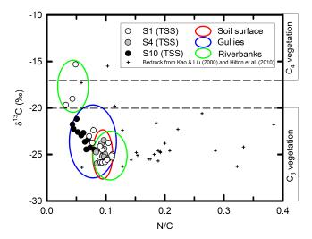
**Figure 6.** Plot of  $\delta^{13}$ C vs. TN / TOC for total suspended sediment loads (TSS) collected at S1 (open circles), S4 (grey circles) and S10 (closed circles) during the 23 May 2012 flood and for the potential sources of sediment (Soil surface: red area; Gullies: blue area; Riverbanks: green areas) determined in the catchment. Bedrock data (plus signs) are taken from the literature (Kao and Liu, 2000; Hilton et al., 2010).
