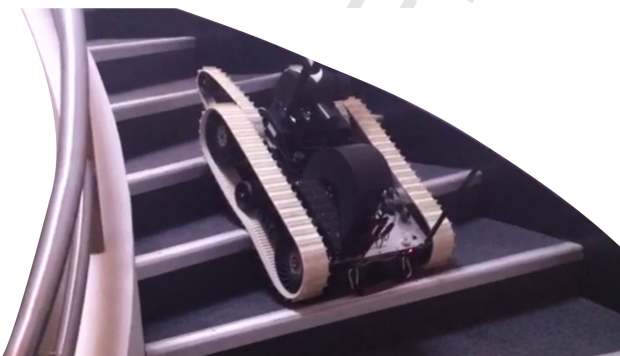
Figure 1: A Cameleon EOD , a tracked mobile robot from Eca Robotics [41]. It consists of one main base, two tracks and two coupled frontal flippers. The details on the robot specification are given in the text.
