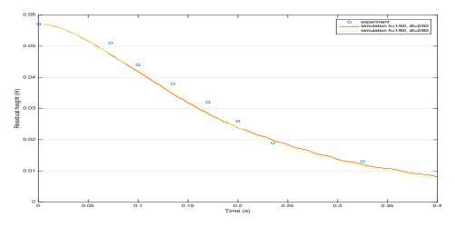
FIGURE 13. Comparison of experimental and approximated height of residual water variation with collapsing time in 3 dimensions.
