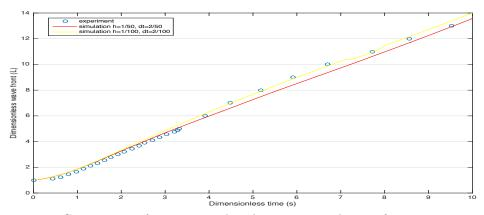
FIGURE 7. Comparison of experimental and approximated wave front variation with collapsing time.
