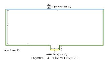
The considered mesh contains 7329 vertices and 14316 triangles where the boundaries  $\Gamma_0$ ,  $\Gamma_1$  and  $\Gamma_2$  are divided into N segments per unit length (where N = 50).
