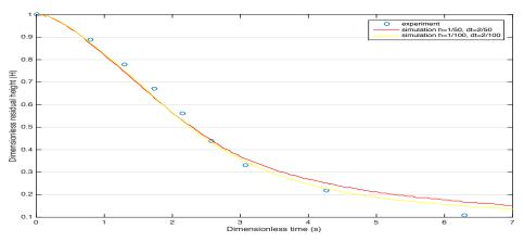
FIGURE 8. Comparison of experimental and approximated height of residual water variation with collapsing time.
