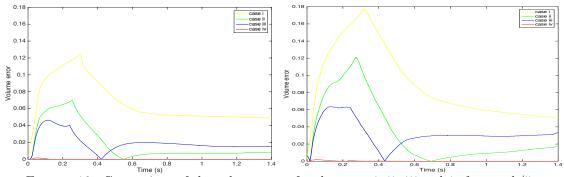
FIGURE 19. Comparison of the volume error for the cases *i*, *ii*, *iii* and *iv* for  $\varepsilon = h/5$ . To the left: classical method; To the right : projection method
