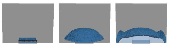
FIGURE 22. The approximated interface at  $t = 0, t = 0.12 \ s$  and  $t = 0.2 \ s$ .
