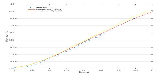
FIGURE 12. Comparison of experimental and approximated wave front variation with collapsing time in 3 dimensions.
