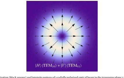
Figure 3. Polarization (black arrows) and intensity pattern of a radially polarized optical beam in the transverse plane z = 0, as described by equation (23).
