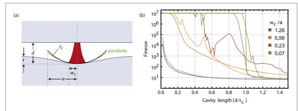
**Figure 6.** (a) Schematic of the cavity showing the relevant parameters. (b) Simulated finesse for different mirror profile size at fixed radius of curvature  $r_c$  using various ratios of  $w_c/a$  defined at  $d = r_c/2$ . Solid lines: Gaussian profile. Dashed lines: parabolic profile. We assume additional loss of  $\pi \times 10^{-7}$  for each mirror.
