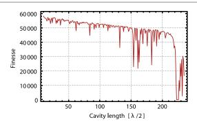
**Figure 2.** Cavity finesse as a function of axial mode order determined from measurements at 25 different positions within an area of  $30 \times 30 \ \mu m$  on a large planar mirror and taking the most prevalent values. Wavelength: 780 nm.
