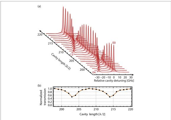
**Figure 4.** (a) Measured cavity transmission spectra as a function of relative cavity detuning. Wavelength: 856 nm. Avoided crossings between the fundamental mode and the fourth order modes 04 and 13 are visible. (b) Maximal transmission of each of the spectra shown in (a), normalized to the largest value.
