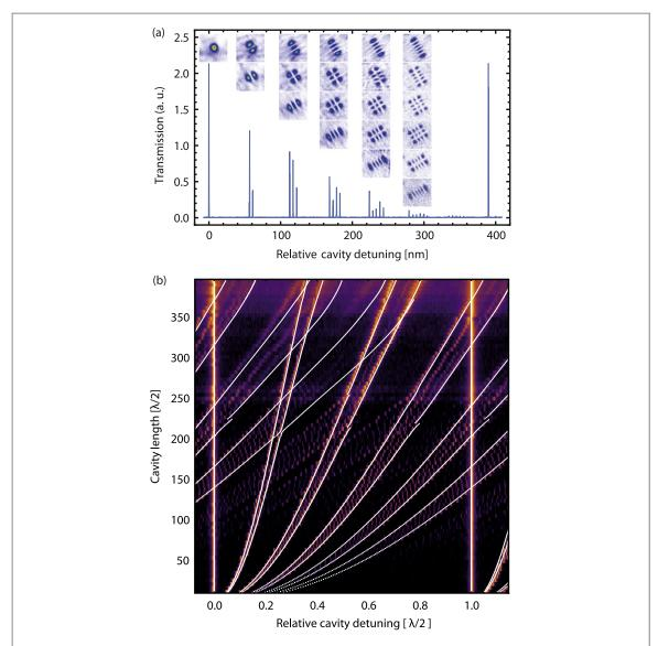
**Figure 3.** (a) Cavity transmission spectrum as a function of relative cavity detuning covering one free spectral range, where  $\mathcal{F} \approx 60.000$ . The insets show the mode functions as measured by scanning cavity microscopy. Wavelength: 780 nm. (b) Cavity transmission spectra as a function of axial mode order q for  $\mathcal{F} \approx 1200$ . Logarithmic color scale. Wavelength: 856 nm. White: model for modes (0, m+n) and (m+n, 0).
