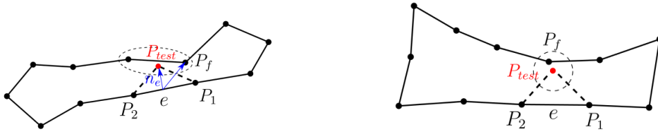
Figure 20: Planar schematics of two criteria for checking if P_{test} is suited as a new vertex of the mesh: point-edge criterion (left) and distance criterion (right).
