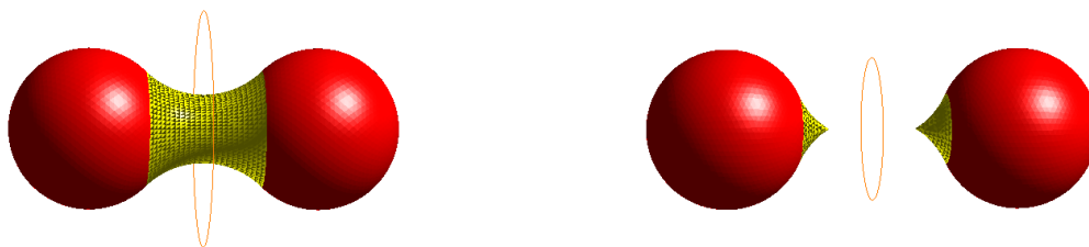
Figure 5. Schematics of a rectangle-shaped toroidal patch (left, yellow) and a double-triangle-shaped toroidal patch (right, yellow) corresponding to two circular SAS circles respectively with radius larger than and smaller than r_p .
