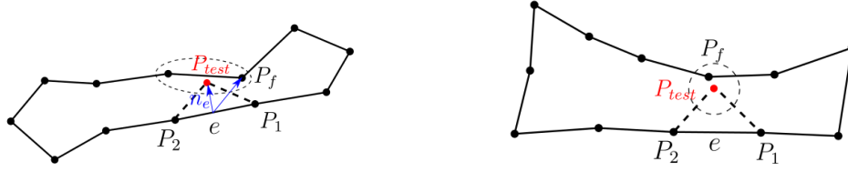
Figure 8. Planar schematics of two criteria for checking if P_{test} is suited as a new vertex of the mesh: point-edge criterion (left) and distance criterion (right).
