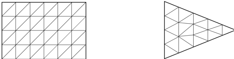
Figure 11: Schematics of meshing a rectangle (left) and an isosceles triangle (right) with the boundary division given.
