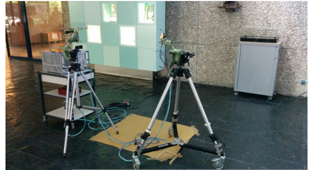
Fig. 5: VNA-based measurement set-up.
