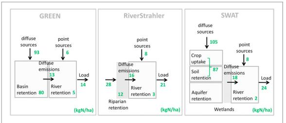
**Figure 6.** Nitrogen fluxes and retention in the Seine river basin according to the three models considered in this study: GREEN (left), RiverStrahler (centre) and SWAT (right). Values are expressed in kgN  $\,\mathrm{ha}^{-1}$  and are annual average values for 1995–2005.
