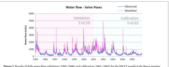
**Figure 2.** Results of daily water flow validation (1995–2000) and calibration (2001–2005) for the SWAT model at the Poses gauging station (blue, observed values; pink, the model simulation).
