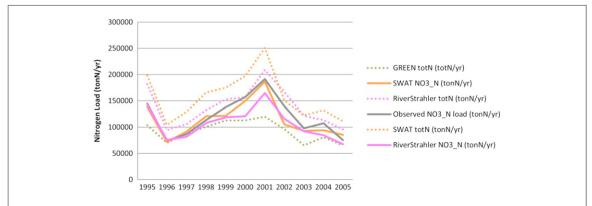
$\textbf{Figure 4.} \ Simulation \ of annual \ nitrate \ (NO_3) \ and \ total \ nitrogen \ (totN) \ loads \ observed \ (grey) \ and \ simulated \ by \ the \ GREEN \ (green), \ RiverStrahler \ (pink) \ and \ SWAT \ (orange) \ models, \ at the \ Poses \ gauging \ station.$
