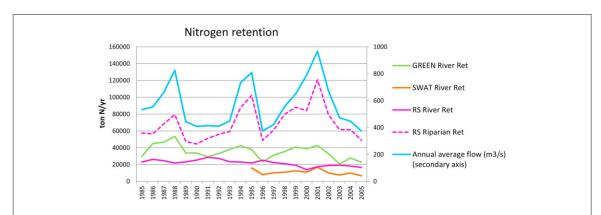
**Figure 7.** Temporal variation of river nitrogen retention (tonN yr $^{-1}$ ) estimated by the three models considered in this study: GREEN (green), RiverStrahler (pink) 1985–2005 and SWAT (orange), for 1995–2005 at the Poses gauging station. The secondary axis shows the annual average flow (m $^3$  s $^{-1}$ ).
