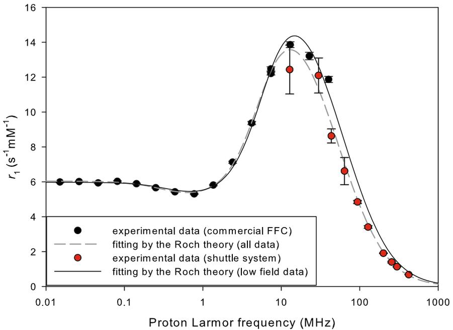
**Fig. 2**  $T_1$  NMRD profile of Gadospin™ at 25 °C
